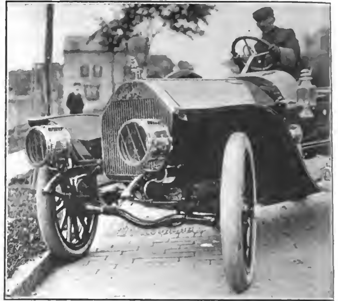
Fig. 2—Another view of the same automobile taken to show how the sharp edge of the curb eats its way into the tread of the tire
